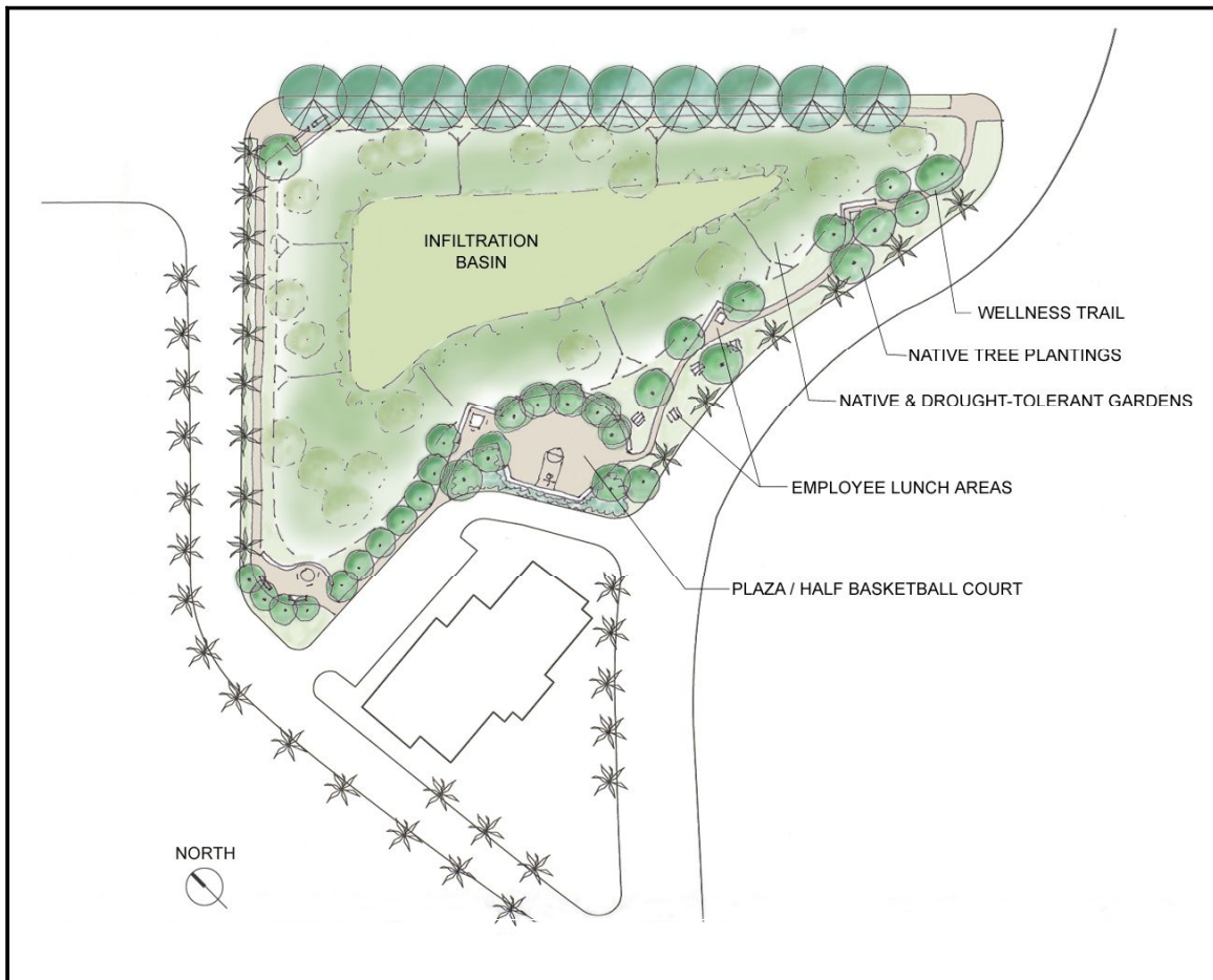
Figure 3-6 Steam Plant Infiltration Basin for Plant Runoff
